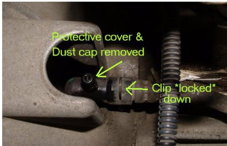
Now pull up the spring clip that holds the feedpipe in place<sup>1</sup>. Gently pull the feed pipe out by about 4mm. If this hasn't been done for a while try gently twisting the pipe as you pull to release it (holding the metal end, not the rubber pipe!). If you have a clear bleed pipe you will probably see the fluid start to flow.
