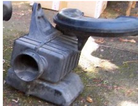
Remove two 10mm bolts at the back of the air box holding it to a bracket under the battery tray. The bracket should be bolted to the front of the tray and also has a clip that takes some of the wiring. Then lift it out upwards, especially if you have air conditioning as the pipes get in the way.
