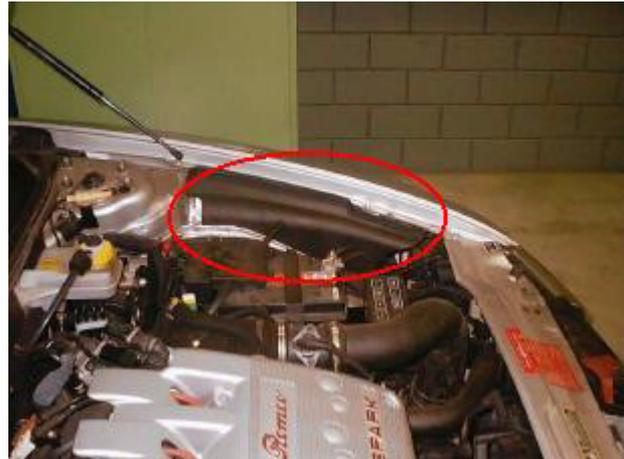
Now the fun bit! Take the intake box with two hands to pull hard to get it out of the air filter housing. This can be difficult (to say the least!). Use a screwdriver to lever the parts apart if necessary. It should be easier if you leave the airfilter box bolted in place, but you can loosen the air filter housing to get more room and allow you to twist them apart. Watch closely how the filter box is installed so you can reinstall it in the same way.
